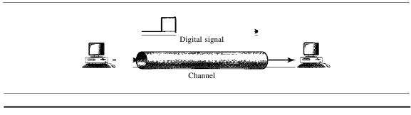
A digital signal is a composite analog signal with an infinite bandwidth.
