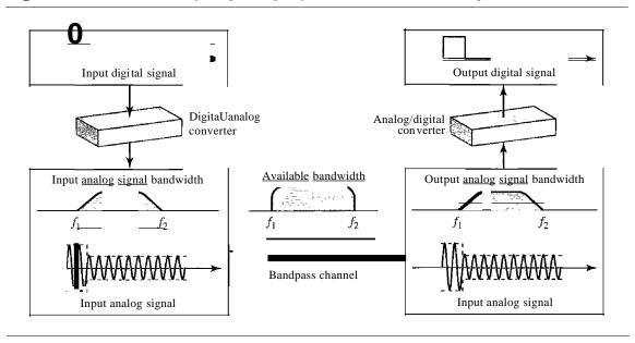
Figure 3.24 Modulation of a digital signal for transmission on a bandpass channel
