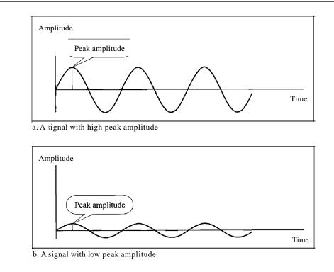
This discrepancy is due to the fact that these are root mean square (rms) values. The signal is squared and then the average amplitude is calculated. The peak value is equal to  $2^{112}$  x rms value.
