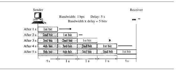
Figure 3.31 Filling the link with bits for case 1
