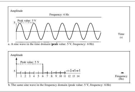
It is obvious that the frequency domain is easy to plot and conveys the information that one can find in a time domain plot. The advantage of the frequency domain is that we can immediately see the values of the frequency and peak amplitude. A complete sine wave is represented by one spike. The position of the spike shows the frequency; its height shows the peak amplitude.
