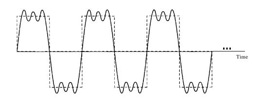
It is very difficult to manually decompose this signal into a series of simple sine waves. However, there are tools, both hardware and software, that can help us do the job. We are not concerned about how it is done; we are only interested in the result. Figure 3.10 shows the result of decomposing the above signal in both the time and frequency domains.
